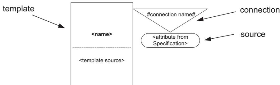
Fig 7: Elements of Configuration Diagram
